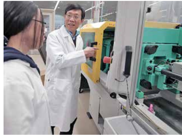
Professor Lih-Sheng (Tom) Turng and Emily Yu, a postdoctoral research associate in Turng's lab, brainstorming next to a micro-injection molding machine capable of mass producing plastic and composite parts with microscale dimensions or geometric features suitable for tissue engineering applications.
