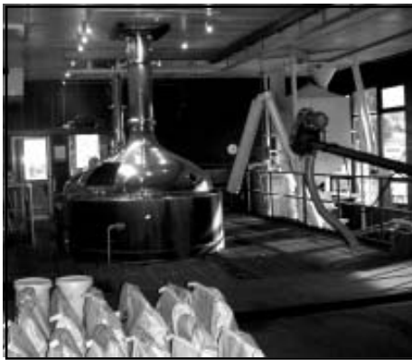
A copper brewing kettle at Capital Brewery in Middleton, WI.
