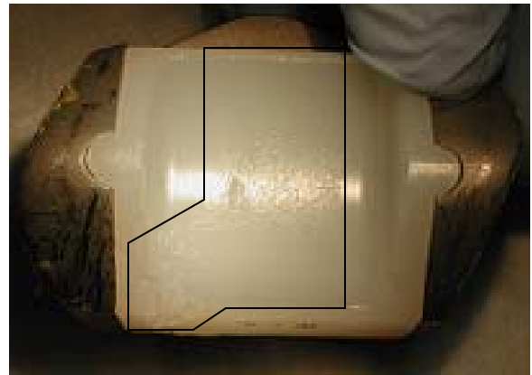
Figure 5: Typical wear pattern on an AGILITY clinical retrieval
