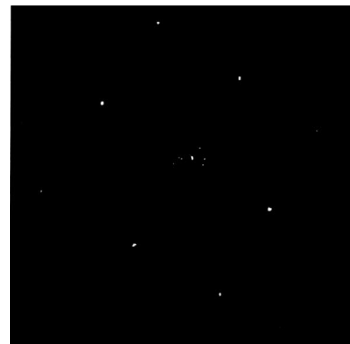
Fig. 5. Optical diffraction pattern of the two-dimensional poled nonlinear photonic crystal.
