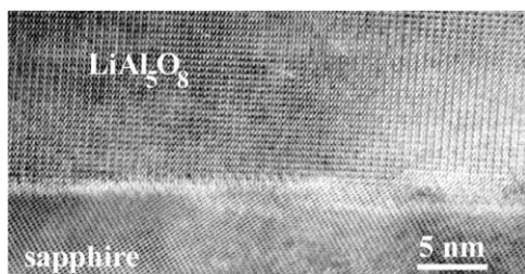
Fig. 6. High-resolution TEM cross-section image of the \text{LiAl}_5\text{O}_8/\text{Al}_2\text{O}_3 interface. The film was grown on [0001] \text{Al}_2\text{O}_3 at 700^\circ\text{C} and annealed for 1 h at 1100^\circ\text{C} .
